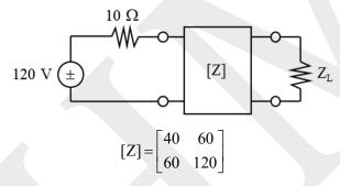
Value of  $Z_L$  for which maximum power is delivered to load is \_\_\_\_\_ $\Omega$
