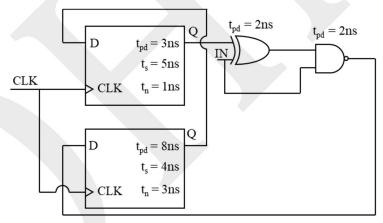
$t_{pd}$  = propagation delay
