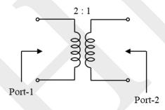
For the above 2-port network consisting of an ideal lossless transformer, parameter  $S_{21}$  for a reference impedance of 10  $\Omega$  is \_\_\_\_\_ (2 decimals).
