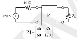
Value of  $Z_L$  for which maximum power is delivered to load is  $\Omega$
