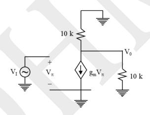
$$\frac{V_{o}}{V_{t}} = -g_{m}.5k = -89.42$$
