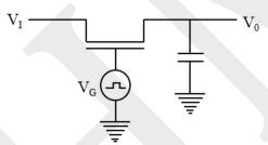
$V_{TH} = 3\ V,\ V_{SUB} = -10\ V,\ V_I: (-10\ V,+10\ V)$  minimum and maximum values of  $V_G$  for proper sampling and holding respectively are
