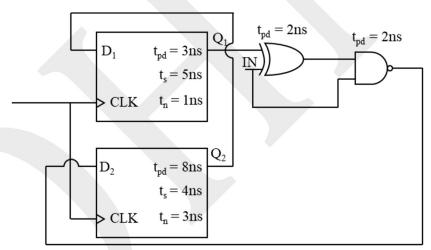
The logic in this question is "the data at the input of one of the FF should arrive at the next FF t<sub>s</sub>(setuptime) (of second FF) before next active edge of clock"
