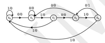
For the above FSM, the sequence that is being detected is input bit pattern until output is 1 [on arrows the format is input/output].
