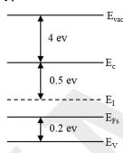
$$E_g = 1 \text{ ev; } V_{TH} = -0.16 \text{ V}$$
