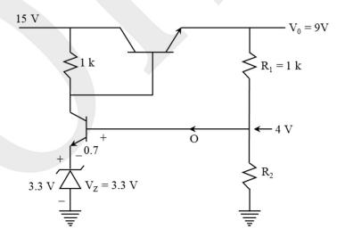
$$\frac{G \times R_2}{R_1 + R_2} = 4V$$
