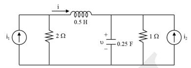
Which is the correct state equation for the above circuit?
